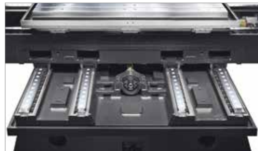
The bed uses four linear guide ways design ( AF-1400 / AF-1600 / AF-1800 )
