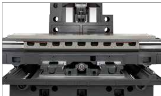
Compound six guide ways base ( BM-2100 / BM-2500 )
