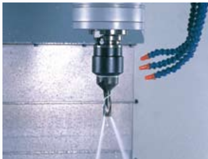
Coolant Through Spindle System ( Opt. )
