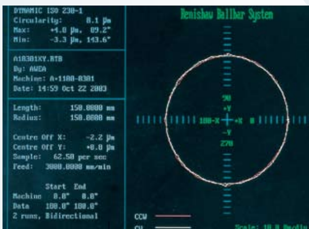
BALL BAR INSPECTION
